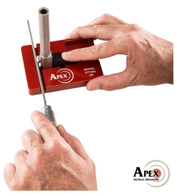
Using the Apex Barrel Fitting Jig to fit the Bottom Lock-up Surface
