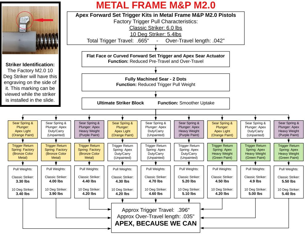
Trigger pull weights are approximate and can vary based on factory tolerances. Our measurements were taken with a "Trigger Scan" machine which pulls the trigger mid line between the Safety Pivot Pin and trigger quard. Your results with a manual trigger pull gauge will likely vary(lower than our readings) if you pull the trigger at the lowest point possible.
